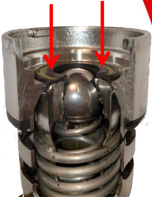
Cracked rubber from UV exposure (sunlight)
