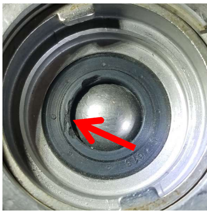
Impact damage to raised rim on CO 2 Valve
