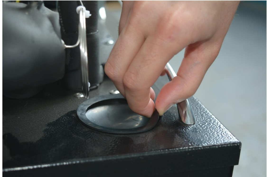
Fig. 6 - Removing the cap to fill the glycol
