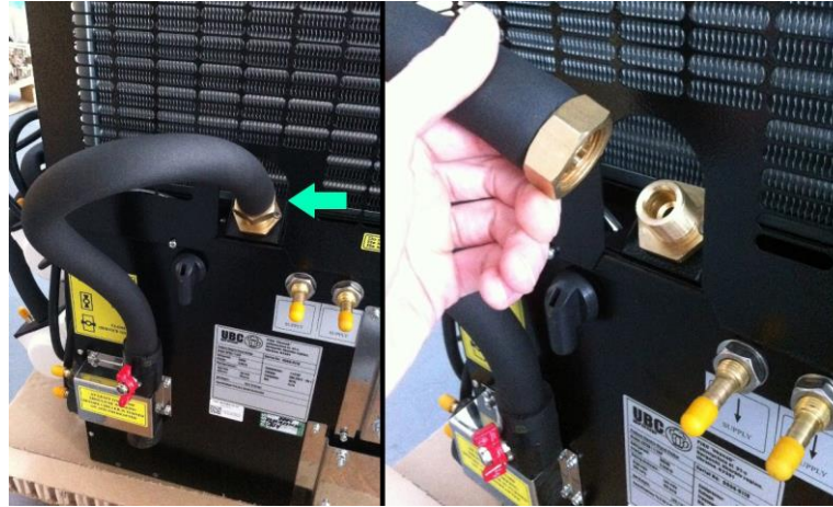
Fig. 8 - Disconnecting the glycol return hose
