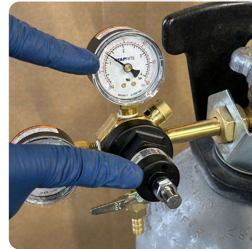
Set CO2 to 30 PSI or higher, as per beer pressure guide
