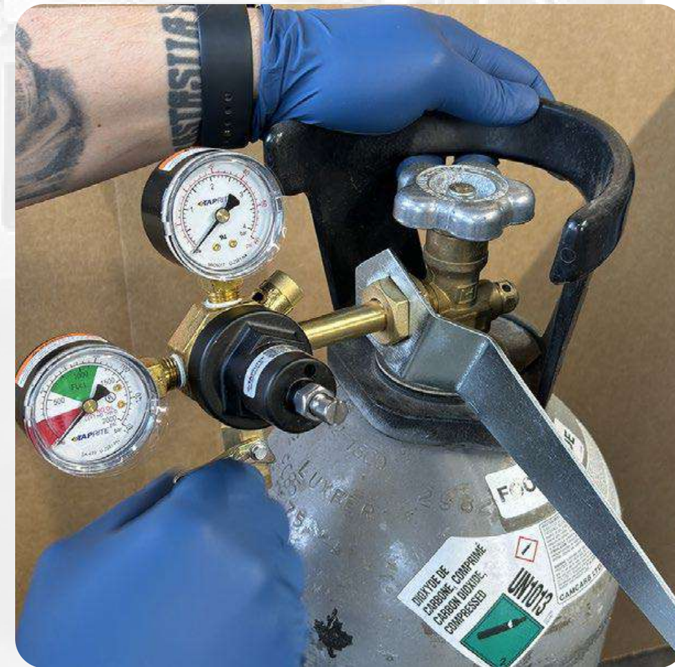
Use CO2 regulator in CLOSE position
