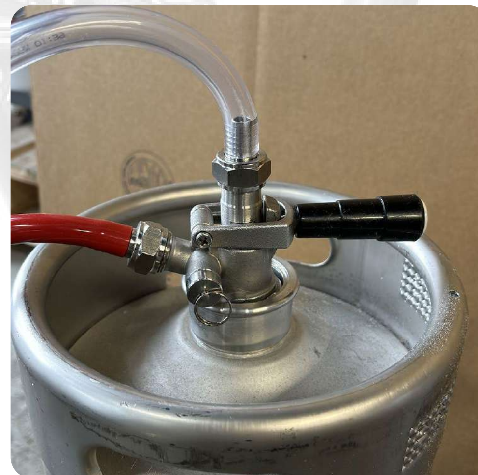
With black coupler handle down the coupler is now engaged. CO2 pressure from the keg should start to push beer throughout the system.
